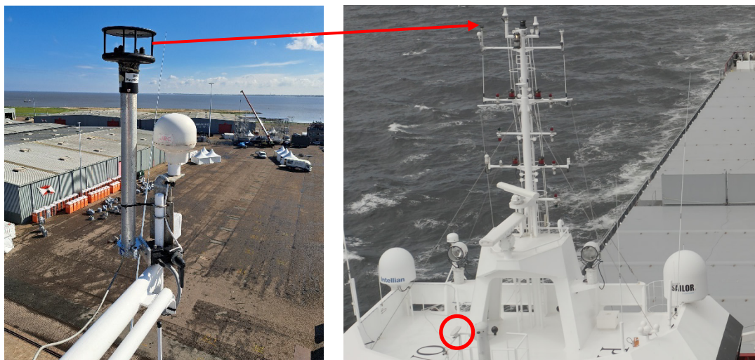
Figure 2-1: Ultrasonic anemometer installed in the ship's mast, and twin D-GPS (encircled) installed on the bridge top
